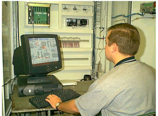
McGill AirClean Service Engineer and PC-HMI interface.
