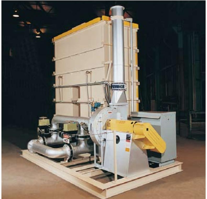
*ThermaGrid RTO systems for smaller volume flows (1,000 to 9,000 scfm) are skid-mounted and electrically heated, making them easy to install or move to various locations. This system for an asphalt loading station (volume flow: 1,000 scfm) controls heavy hydrocarbons, methane, heavy oils, and H<sub>2</sub>S emissions.*
