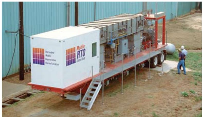
*McGill can use one of our mobile RTOs to perform a pilot test program at your facility to demonstrate the feasibility of using a full-scale RTO to control your emissions.*
